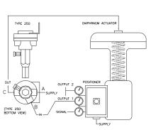
To adjust the cut-off set point, remove the cap and adjust the spring adjusting screw until desired outlet cut-off pressure is achieved. Turning the adjusting screw clock-wise will increase the cut-off setting and turning it counter-clock wise will reduce the cut-off setting. Note that the lock-up relay has a differential pressure of 2.5 psig (.17 BAR). Replace cap securely after having re-adjusted the cut-off set point.
